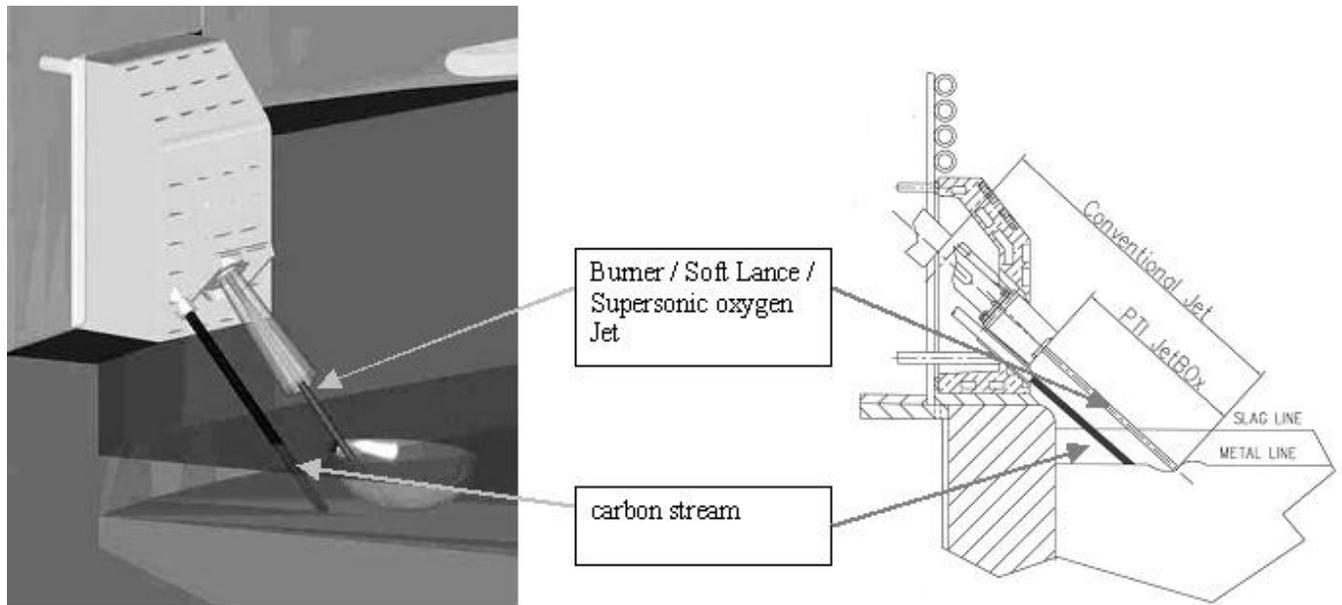
The copper box is designed for long life, with the ability to withstand the impact of falling scrap, while at the same time provide excellent cooling. The box is located just above the last course of
