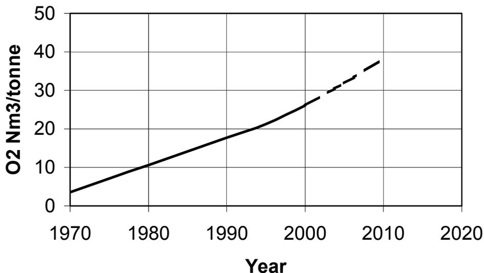
Over the same period of time average transformer power has increased and tap-to-tap times have dropped considerably. This reduces the time available for efficient oxygen introduction and places higher demands on the new chemical energy system and it's operation. Significantly larger amounts of oxygen need to be injected per time unit and efficiency of this energy introduction plays a greater role in overall furnace efficiency.
