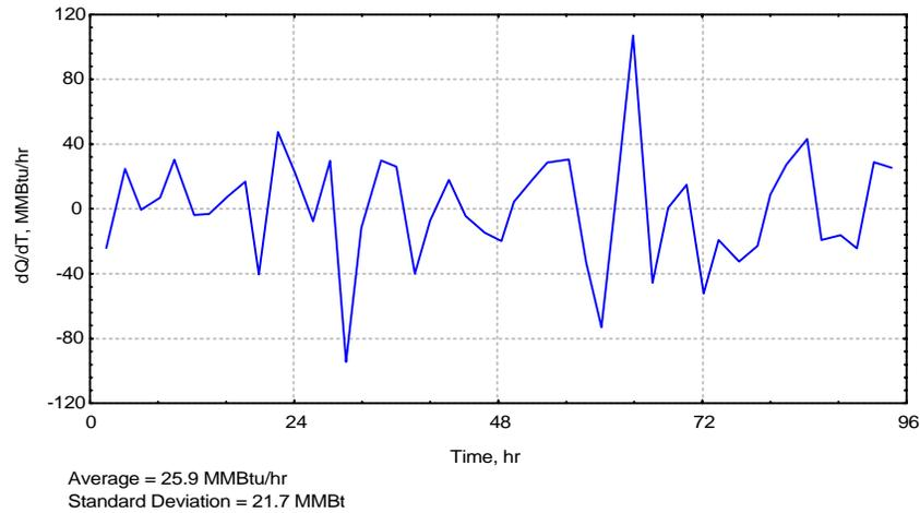
**Figure 7-16B. Cast-to-Cast Variations in the Hearth at Acme: Phase A, Period 3, 147 Ib/THM Natural Gas Injection Rate**
