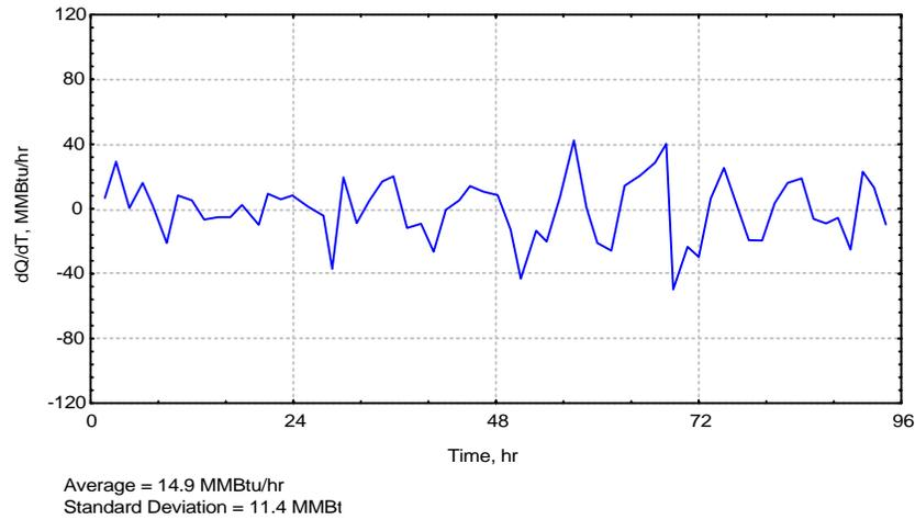
**Figure 7-16D. Cast-to-Cast Variations in the Hearth at Acme: Phase C, Period 1, 232 Ib/THM Natural Gas Injection Rate**
