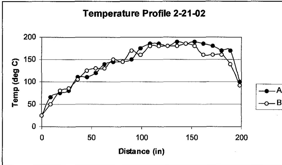
Figure 13 Temperature Profile of Tumbling Cocoa Beans in Predryers A and B measured on 2/21/02
