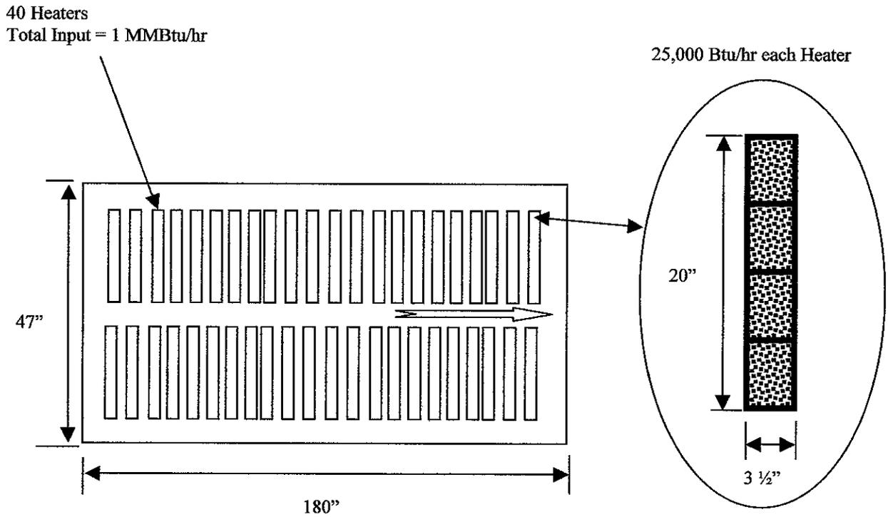
Figure 3. Schematic of the Existing Gas IR Heating System in the Predryer
