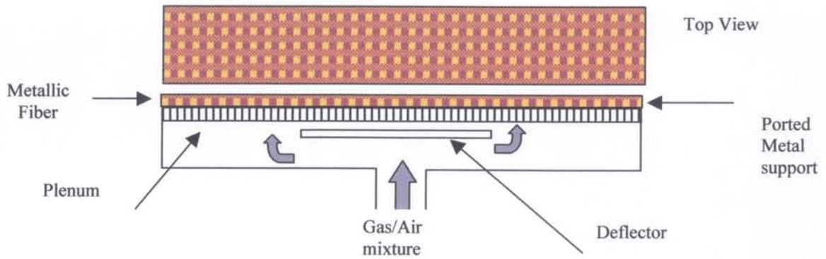
Figure 7. Metal Fiber Surface Combustion Burner
