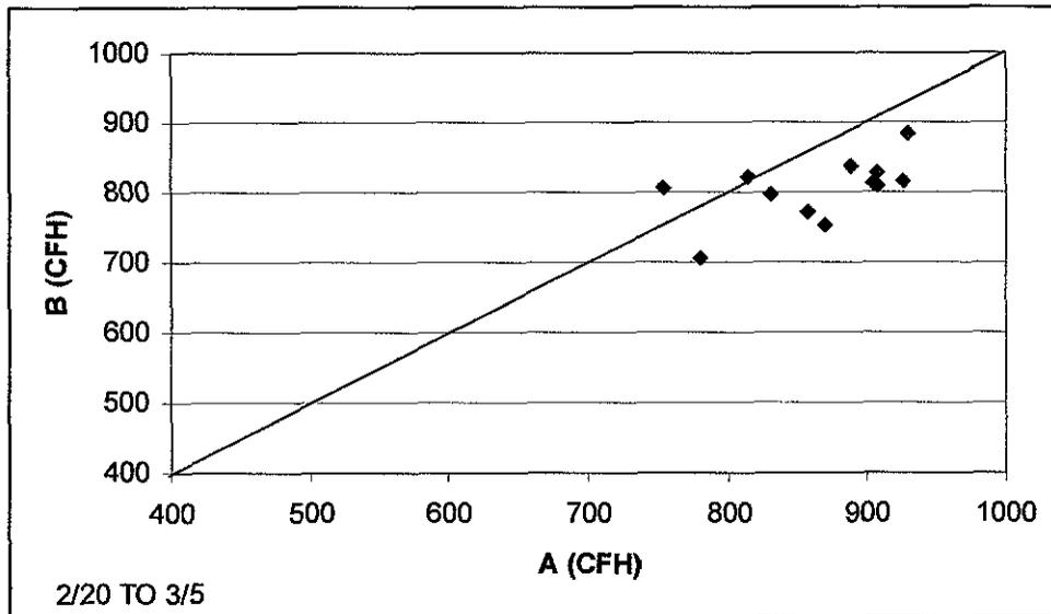
Figure 12 Gas Usage in Predryers A and B from Feb 20 to March 5.
