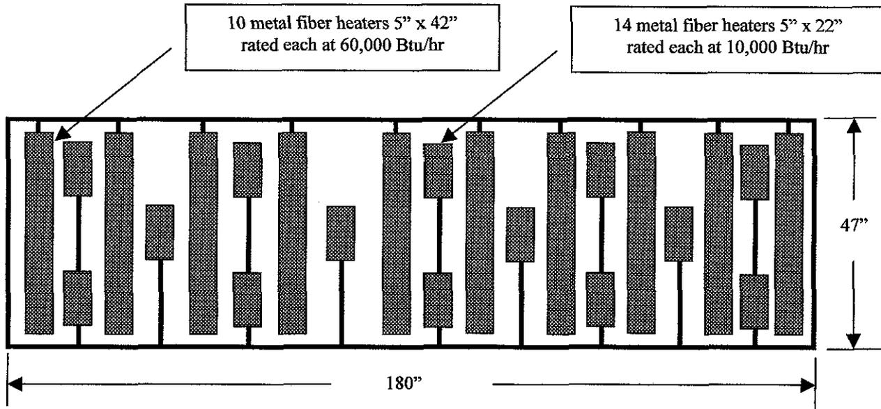
Figure 10. Schematic of IR heater arrangement
