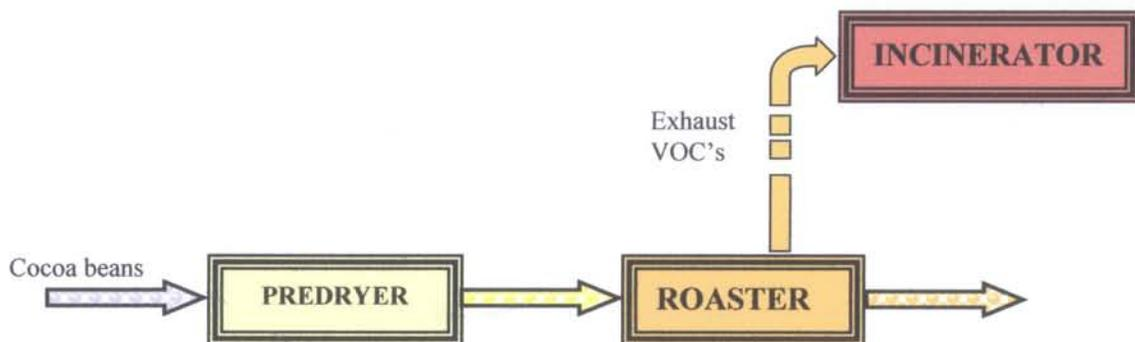
Figure 1. A Schematic of Process Flow through Predryer, Roaster and Thermal Oxidizer
