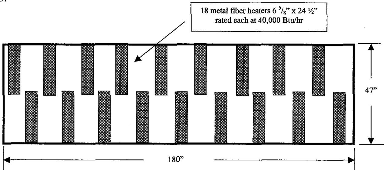
Figure 9. Schematic of IR heater arrangement – Option II
