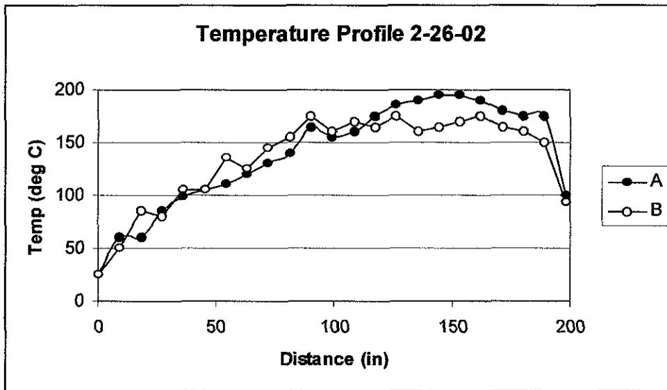
Figure 14 Temperature Profile of Tumbling Cocoa Beans in predryers A and B measured on 2/26/02
