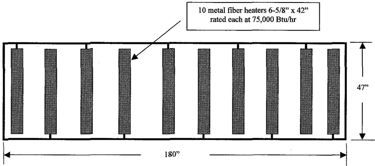
Figure 8. Schematic of IR heater arrangement – Option I
