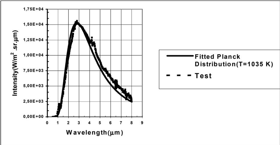
**Figure 15. Spectral Intensity of a Typical Metal Fiber Heater (10 kBtu/hr.ft<sup>2</sup>, 10% Excess Air)**
