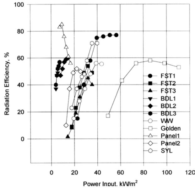
**Figure 7. Radiant Efficiencies of Electrical Heaters**
