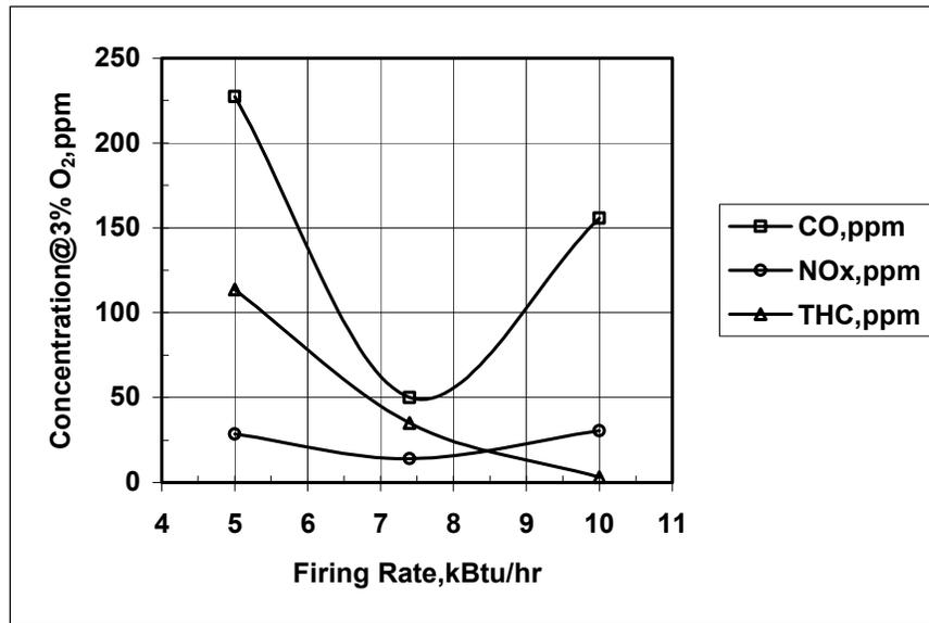
**Figure 17. Emissions Analysis of a Typical Metal Fiber Heater**
