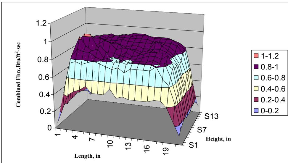
**Figure 14. Radiant and Combined Heat Flux Distributions of a Typical Catalytic Heater.**
