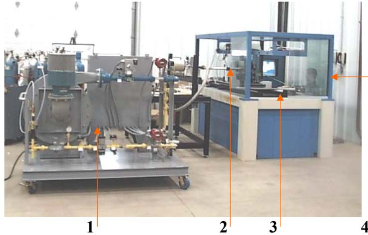
**1. Combustion Rig; 2. Sensor Tube Assembly; 3. Optical Table; 4. Enclosure System**
