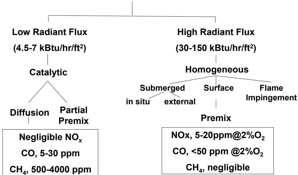
Figure 5. Types of Gas Fired Heaters
