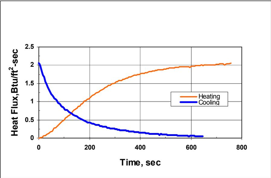
**Figure 16. Heat-up and Cool-down Times of a Typical Electric Heater (1000 Watts)**
