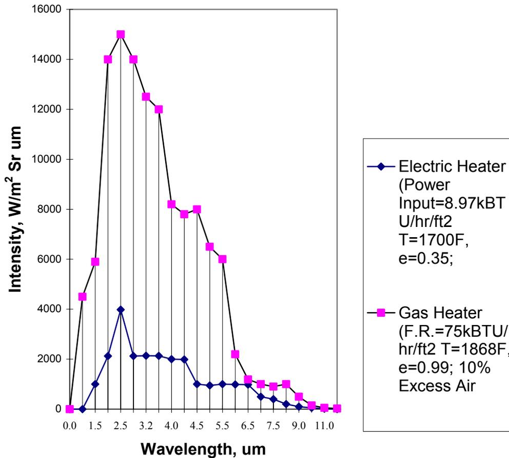
**Figure 9. Comparison of Spectral Intensities of Typical High Flux Gas and Electrical Heaters**
