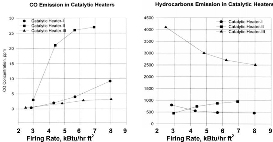
Figure 12. Emissions Analysis of Typical Catalytic Heaters.
