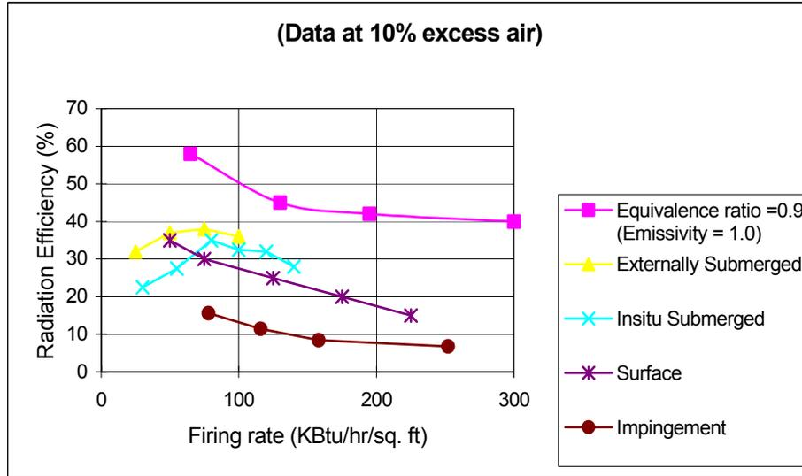
**Figure 6. Radiant Efficiencies of High Flux Gas Heaters**
