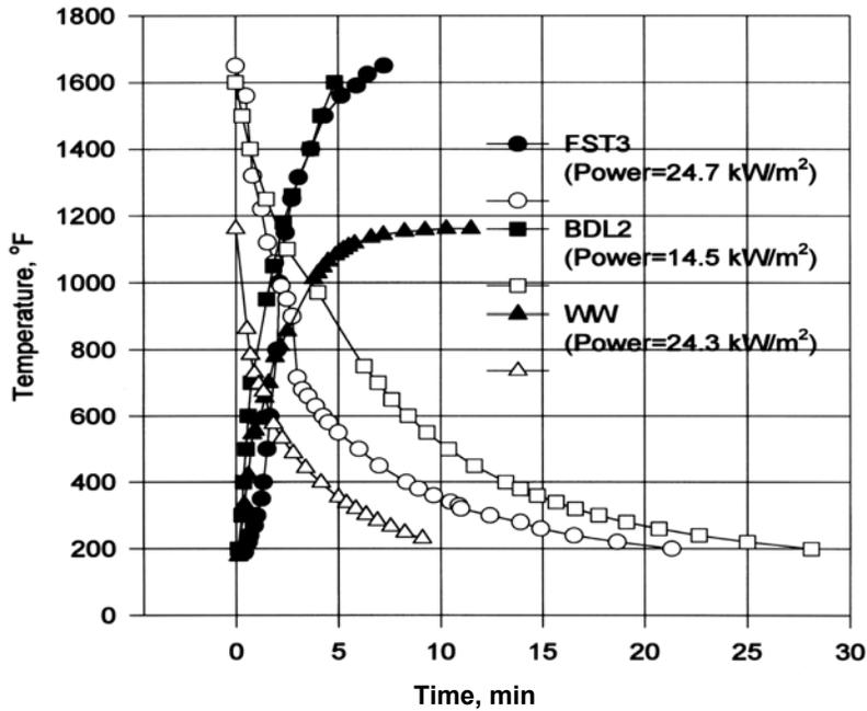
Figure 11. Thermal Response Times for Electrical (Metal Rods/Coils) Heaters.
