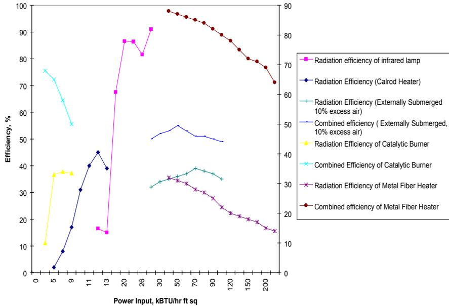
**Figure 8. Comparison of High and Low Flux Gas and Electrical Heaters**
