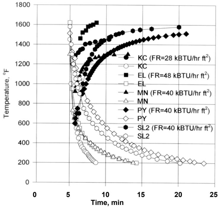
**Figure 10. Thermal Response Times for Typical Surface Combustion Gas Heaters.**
