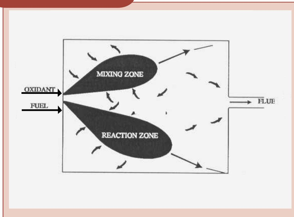
Schematic representation of Dilute Oxygen Combustion.
