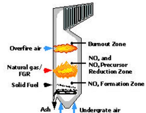
*Methane de-NOX Process Schematic*
