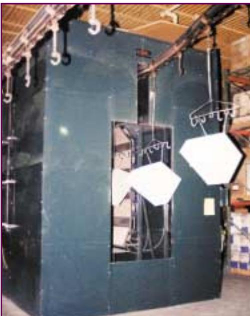
*Designed and engineered by Vulcan Catalytic Systems, Progressive's 40-foot catalytic infrared booster oven was installed between their powder coating booth and the convection oven.*
